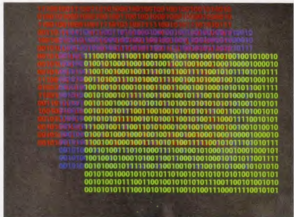
Bitplanes are best thought of as pages in memory - the first bit on each plane contains colour information for the first pixel, and so on.
